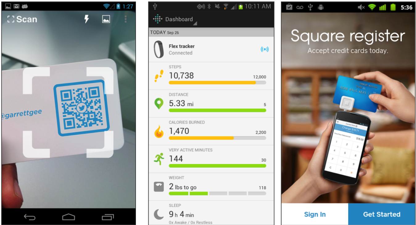
Figure 14: Some apps require special forms of input to trigger app behavior. This figure presents several such examples (right to left): QR Code Reader, Fitbit, and Square. Traversal of these apps may require human intervention or software to emulate the input.
