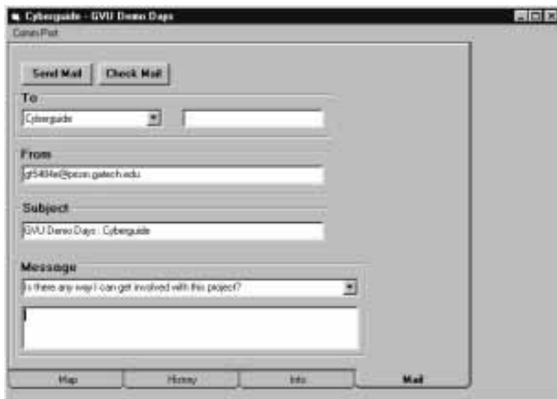
Figure 8: The mail interface of the PC Cyberguide. Addresses are automatically filled in and message templates are supplied upon request.
