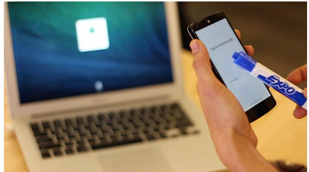
Figure 1. With Thumprint, groups of users learn a single, shared secret knock that they enter on a surface instrumented with (or containing) an accelerometer and microphone (here, a smartphone) in order to authenticate.
